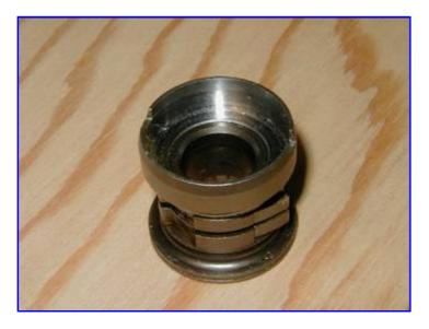
A sealed bearing can be used. Heat the main bearing to remove the hardness, and then machine to  $\sim$ 1.02" inner diameter. A sealed bearing would slightly reduce the width of the freewheel.
