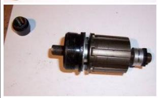
Add the BB cup, a couple more washers, and a nut. Tighten to a torque of one grunt.
