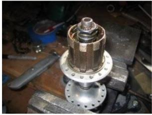
First remove the gear cluster assembly. You may need the special Shimano cluster too to accomplish this, as well as a chain whip tool.
