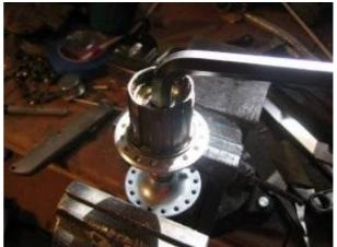
The freehub needs to be taken completely apart so the pals can be removed. This allows will allow the freewheel to spin in either direction.
