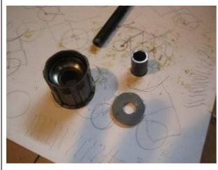
tool or dremel rather than a hacksaw, as the hollow nut is made of hardened steel. Make a thick washer, which will go on the bottom of the freehub.
