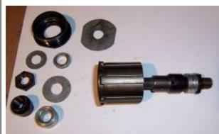
Slide the axle with the "item 4" sleeve into the carrier. An axle nut and a spacer and another nut are to the right of the sleeve. The additional spacer and sleeve will be used to mount the derailleur later.
