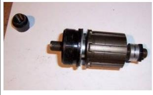
Add the BB cup, a couple more washers, and a nut. Tighten to a torque of one grunt.
