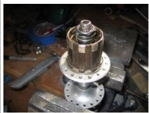
First remove the gear cluster assembly. You may need the special Shimano cluster too to accomplish this, as well as a chain whip tool.
