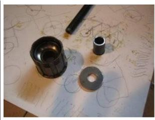
the hollow nut is made of hardened steel. Make a thick washer, which will go on the bottom of the freehub.
