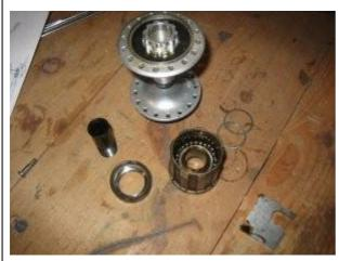
Here's the hub with the hollow bolt, and the bearing cup removed.
