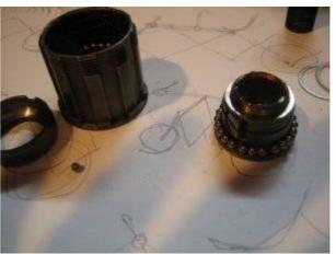
Cut the threaded section off of the hollow bolt. It will be used as a spacer. You will need to use a cut off tool or dremel rather than a hacksaw, as
