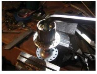
The freehub needs to be taken completely apart so the pals can be removed. This allows will allow the freewheel to spin in either direction.
