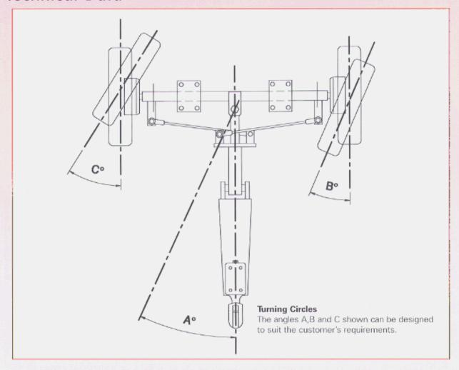
The above track rods are crossed over enabling true Ackermann principle to be achieved, i.e. inner wheel has a greater steering angle than outer wheel, which minimises the tyre wear and promotes trailer stability.
